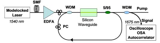
Fig. 2. Experimental set up used for silicon Raman laser demonstration. A ring cavity configuration is used as a resonator. A modelocked fiber laser at 1540nm is used as a pump laser. The lasing is obtained at the Stokes wavelength of 1675 nm.
