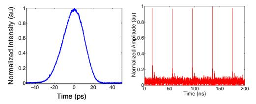
Fig. 5. Measured temporal profile of the laser output. (a) 25 ps pulse trace obtained by an autocorrelator at 1675 nm. (b) Oscilloscope trace shows 25 MHz pulse train at 1675 nm.
