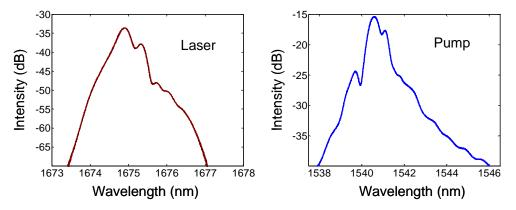
Fig. 4. Measured laser and pump spectra. The laser spectrum has 0.36 nm spectral bandwidth and is located 15.6 THz away from the pump laser. The pump-output separation is precisely the optical phonon frequency in silicon.
