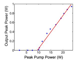
Fig. 3. Measured laser output power with respect to peak pump power. Lasing threshold is measured to be at 9 W peak power level. The slope efficiency is  $\sim$ 8.5%.
