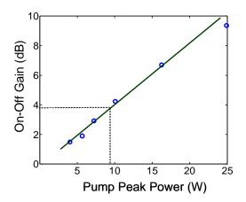
Fig. 1. Measured on-off gain in the silicon waveguide for a probe signal at 1675 nm. Pumping was done at 1540 nm with 30 ps pulses.
